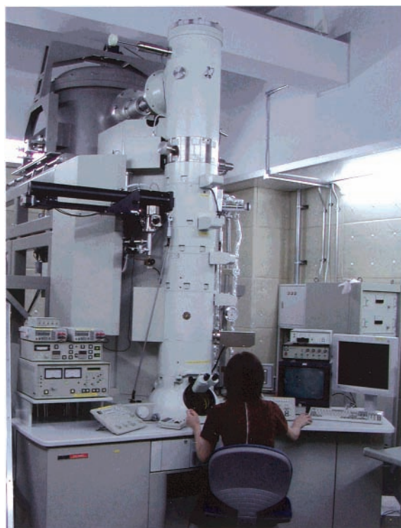
FIGURE 1. A fifth generation electron cryomicroscope equipped with an automatic cryotransfer system, a field emission gun, an omega filter, and a 4K \times 4K slow-scan CCD camera was developed and installed at BIRC, AIST.
